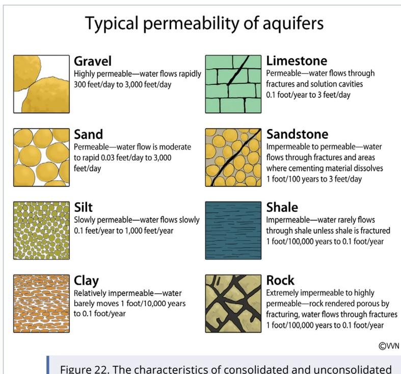
Figure 22. The characteristics of consolidated and unconsolidated aquifers determine the rate at which water can move through them.
