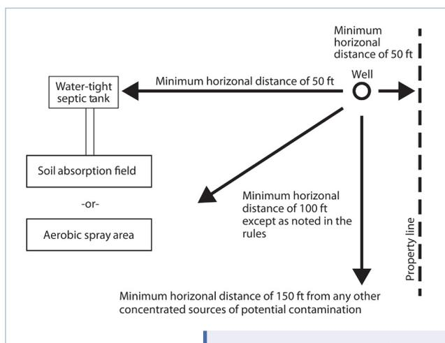
Figure 27. Well location from potential contaminant sources.
