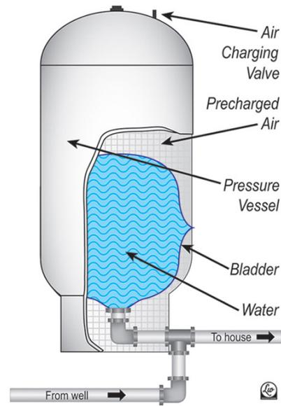
Figure 33. Pressure tank for a private well system. (Source: Gary Hix)
