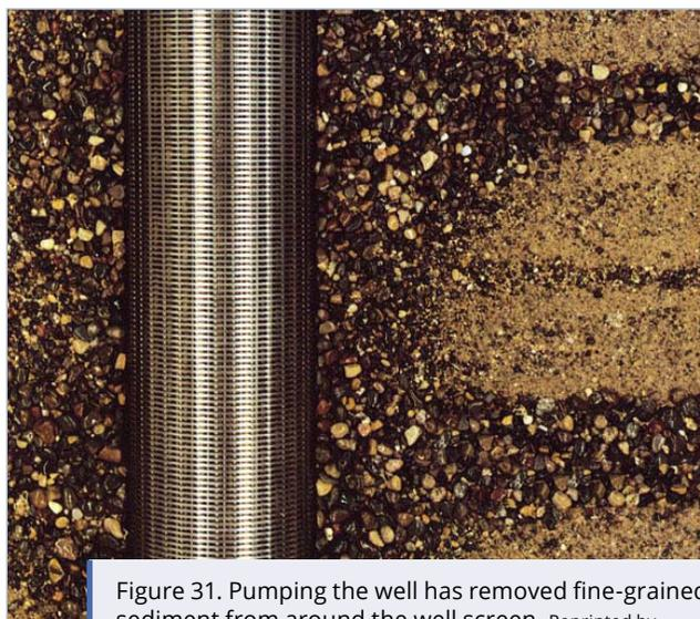
Figure 31. Pumping the well has removed fine-grained sediment from around the well screen. Reprinted by permission of Johnson Screens, a Weatherford Company.
