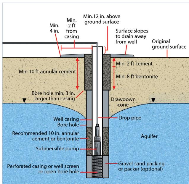
Figure 58. Well construction standards are administered by the Texas Department of Licensing and Registration (TDLR) to protect the aquifer and well from surface water ponding around the well head. Well construction and plugging specifications accepted by the TDLR are shown at <https://www.tdlr.texas.gov/wwd/wwdspecs.htm>.
