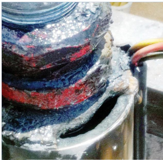
Figure 35. Stray electrical currents formed a hole in this submersible pump. Water was forced through the hole in the bottom of the pump, causing the well screen to collapse and the well system to fail. (Source: Mike Prestigiacomo)
