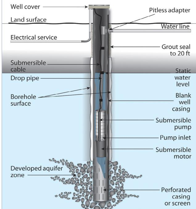
Figure 32. A pitless adapter protects pipes from freezing in cold weather. (Source: Gary Hix)
