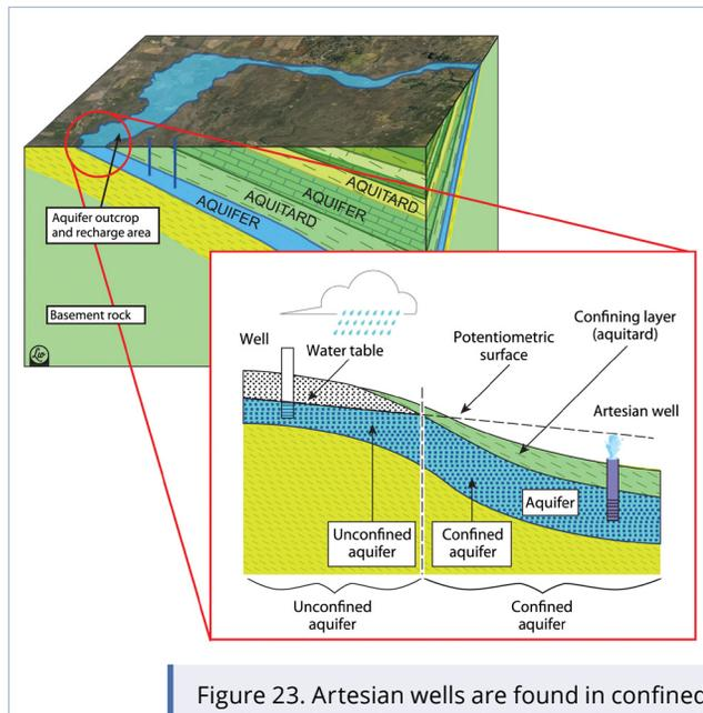
Figure 23. Artesian wells are found in confined aquifers where the water level rises in the well above the confining geological material.
