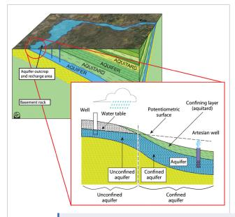
Figure 23. Artesian wells are found in confined aquifers where the water level rises in the well above the confining geological material.
