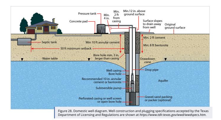
Well casings for household wells can vary from 4 to 8 inches in diameter, depending on the aquifer conditions and the type of pump to be installed. The most common materials for well casings are carbon steel, plastic (usually PVC), and stainless steel. PVC is lightweight, resistant to corrosion, and relatively easy to install.
