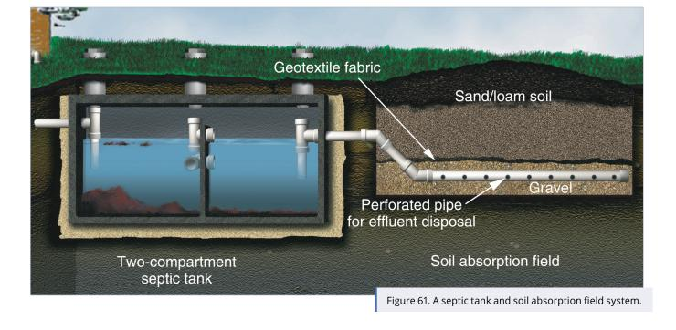
Spent brine discharge from reverse osmosis and water softeners will increase the concentrations of salt in the soil, which could change the soil structure in the leach field and cause the system to fail.
