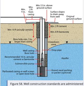
by the Texas Department of Licensing and Registration (TDLR) to protect the aquifer and well from surface water ponding around the well head. Well construction and plugging specifications accepted by the TDLR are shown at https://www.tdlr.texas.gov/wwd/wwdspecs.htm.
