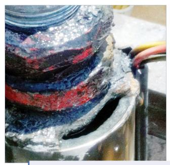
Figure 35. Stray electrical currents formed a hole in this submersible pump. Water was forced through the hole in the bottom of the pump, causing the well screen to collapse and the well system to fail. (Source: Mike Prestigiacomo)
