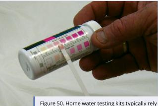
Figure 50. Home water testing kits typically rely on a color change on a test strip to determine the concentration of a contaminant.
