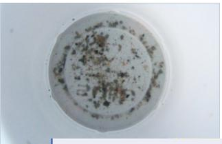
Figure 36. Sand accumulated on the screen of an irrigation system. (Source: Mike Prestigiacomo)
