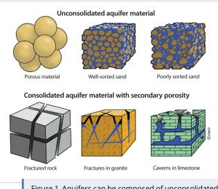
Figure 1. Aquifers can be composed of unconsolidated materials, consolidated materials, or a combination of both.
