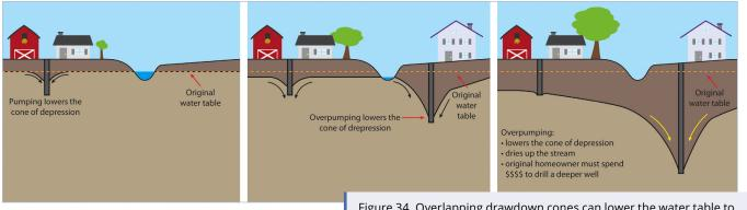
Figure 34. Overlapping drawdown cones can lower the water table to the point where neighboring homeowner wells and rivers can go dry.
