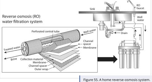
Reverse osmosis is not recommended for pathogens or sediments (particles). For RO to work best, the water should first be pretreated by particle filtration, activated carbon filtration, chlorination, pH adjustment, or even water softening.
